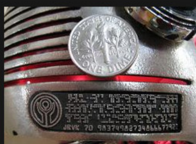
Bar code detail, with dime in place to show size, image courtesy of CCE.
